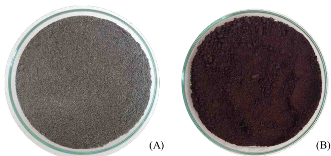
Figure 1: Images of the (A) in natura (LR) and (B) magnetic nanomodified (LR-NP) lettuce roots.
